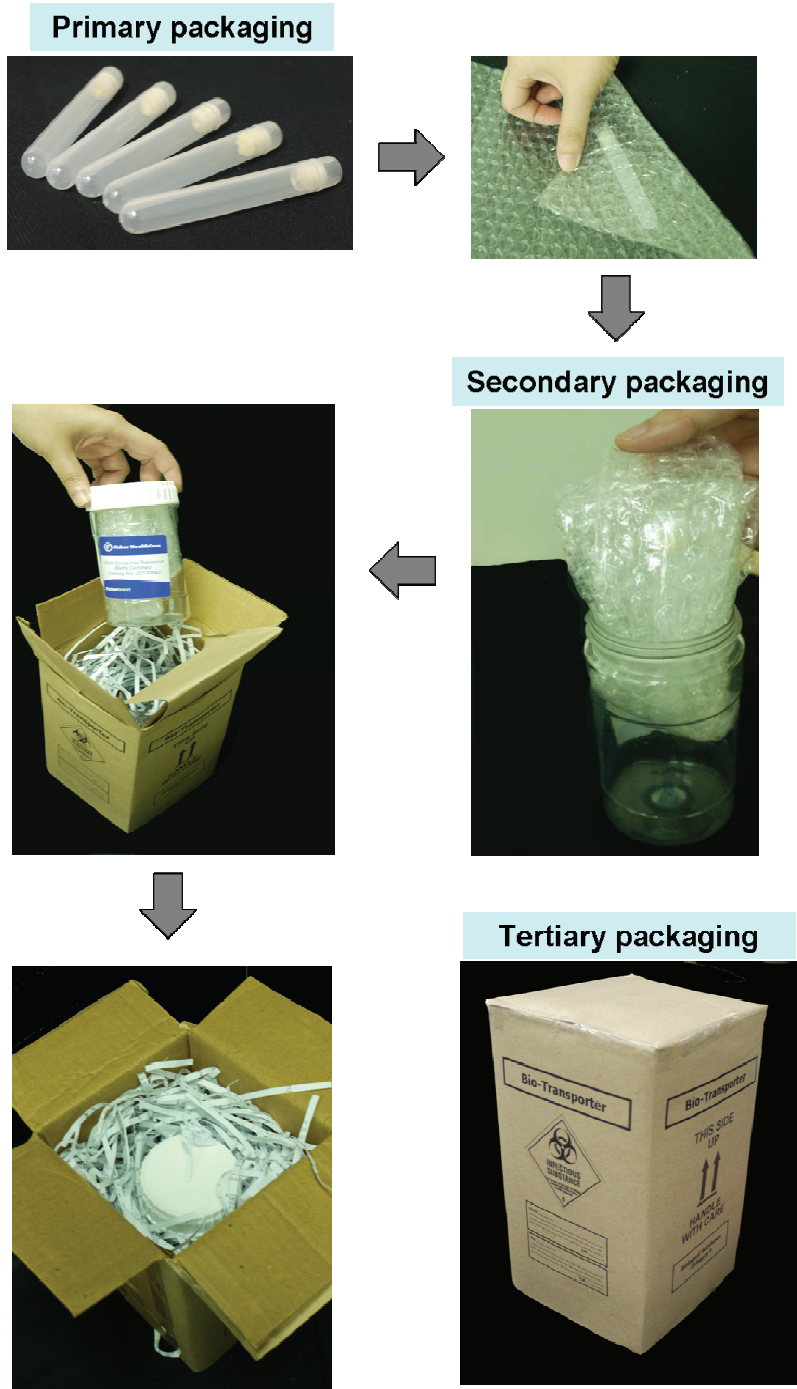
Figure 10.3 Example of the triple packaging system for GMMs (GILSP/class 1) (courtesy of the BIOTEC Culture Collection (BCC), National Center for Genetic Engineering and Biotechnology (BIOTEC), Thailand)
